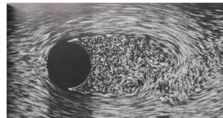
Turbulent wake behind a circular cylinder at Re = 2000 Photograph: ONERA, Werlé & Gallon - 1972 (Van Dyke 1982)
