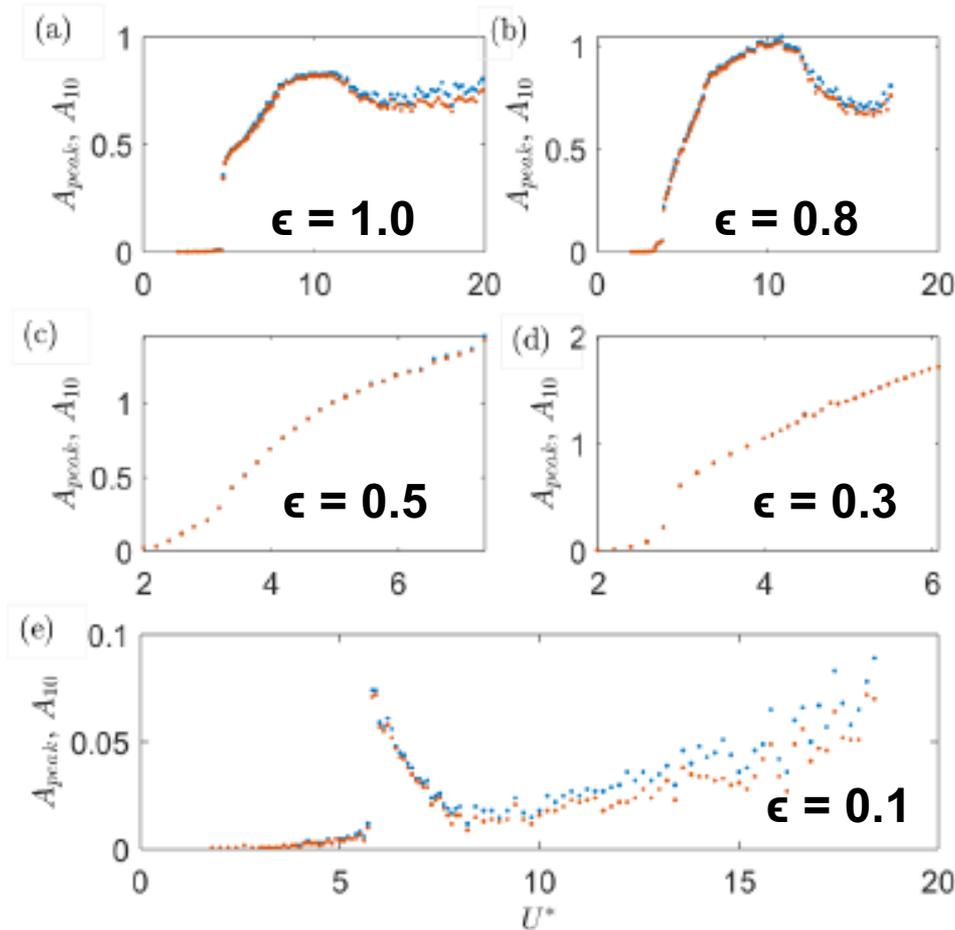
Plots representing the variation between the peak value of vibrational amplitude  $A_{\text{peak}}$  in comparison to the value of  $A_{10}^*$
