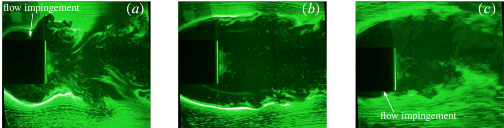
Figure 8: Hydrogen-bubble flow visualisations demonstrating flow impingement in the two synchronisation regions, compared with the negligible vibration region: (a)  $U^* = 3.0$  (Sync-I), (b)  $U^* = 4.0$  (non-vibration region) and (c)  $U^* = 10.0$  (Sync-II) for  $\alpha = 0^\circ$ . See supplementary movies 7 – 9.
