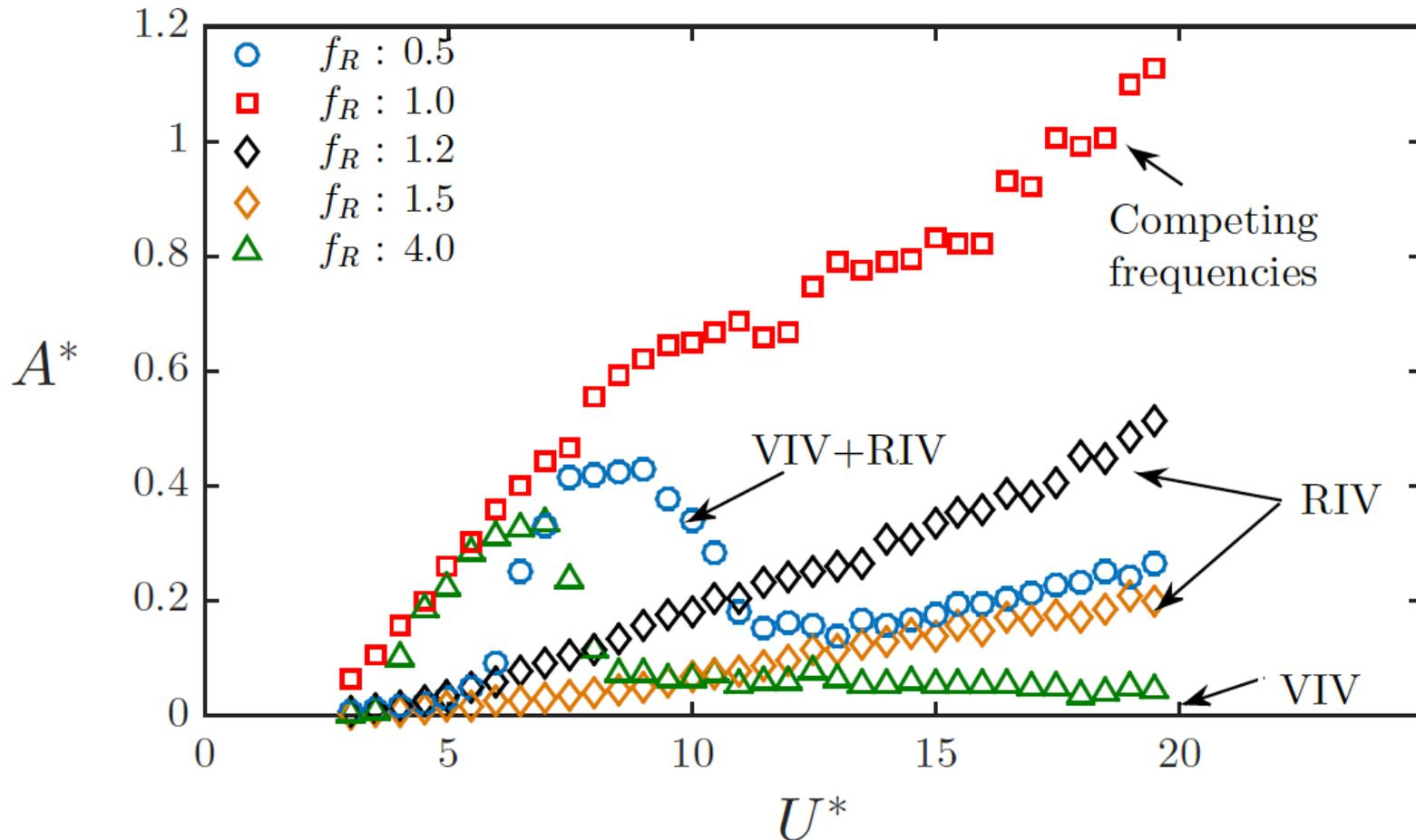
Amplitude response has additional Rotary Induced Vibration (RIV)
