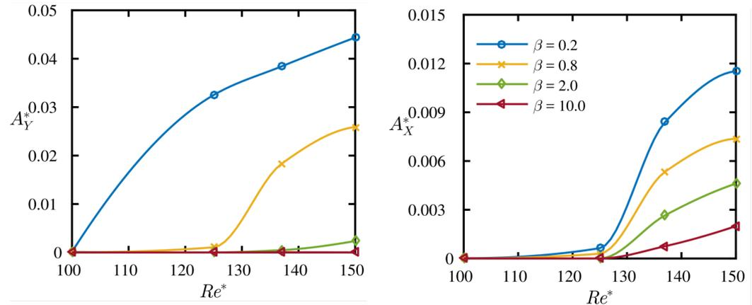
Mean lift and drag coefficients vs  $Re$
