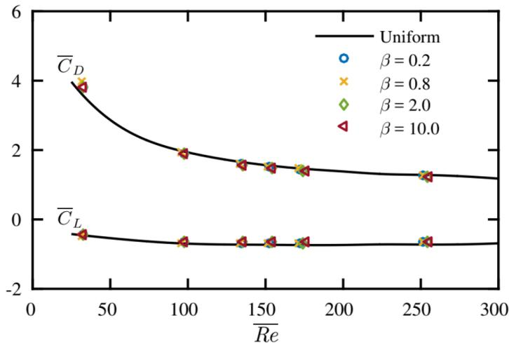
Mean observed drag coefficients vs  $Re$
