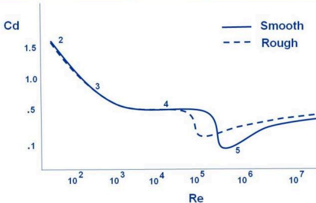
Drag coefficient for flow past a Sphere as a function of Reynolds number  $Re$ . (NASA)
