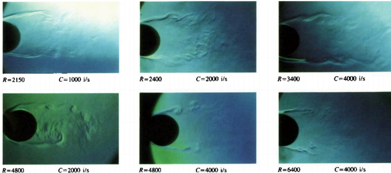
FIGURE 2. Flow visualizations at low Reynolds numbers:  $R=U_0 D/\nu$ ;  $C$ =camera speed in images per s.
