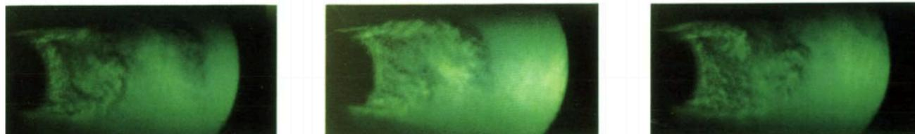
FIGURE 5. Flow visualizations at high Reynolds numbers:  $R=20\ 000$ ;  $C=2000$  i/s.
