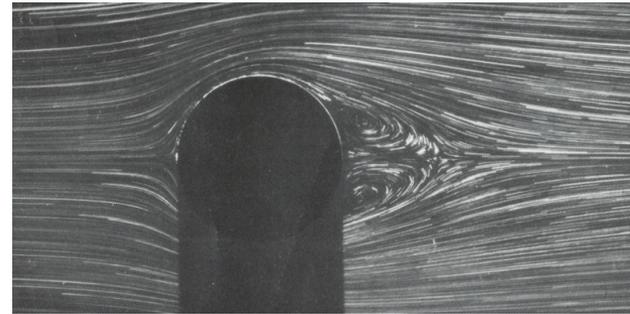
Attached flow (left,  $Re = 0.1$ ) & separated flow (right,  $Re = 56.5$ ) past a sphere
