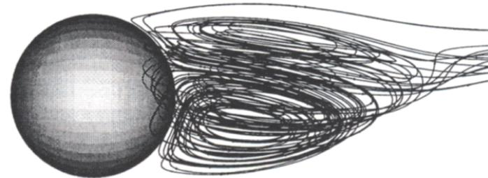
Steady non-axisymmetric wake behind a sphere at  $Re = 250$
